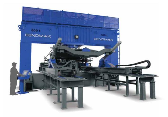
The **DPB-P** models have capacity of power between **150 to 1600 metric** tons and internal distance capacity from **10 to 33 feet**.
